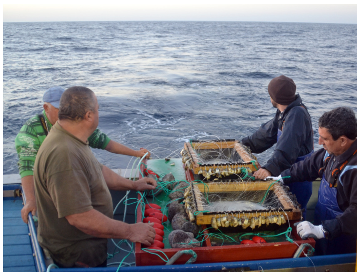
Fig. 4 – Deployment of the long-line at stern of the ship. A metallic table was built in order to allow a safe operation of the long-line.
